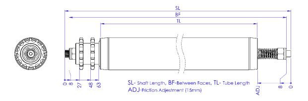
Accumulation Rollers are used to hold or buffer products into areas such as merges, sortation or palletizers. These rollers allow goods stop and accumulate on the conveyor line without stopping the conveyor drive. The AIROLL 60.3 Diameter Accumulation Conveyor Rollers are ideally suited to convey Pallets, Containers or Cardboards.
